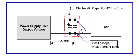
※ Ripple and noise are measured at the end of output cable which are added a 0.1uF ceramic capacitor and 47uF electrolytic capacitor.(connected parallel)
